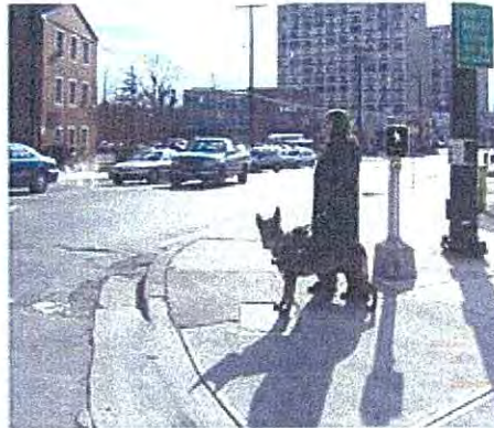
Pedestrian with dog guide at an APS located in line with crosswalk.
