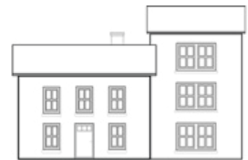
EXISTING HOUSE AND ADDITION WITH INCOMPATIBLE PROPORTIONS
