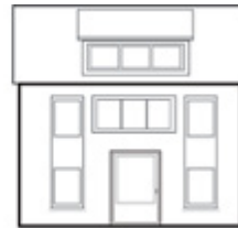
NEW CONSTRUCTION WITH INCOMPATIBLE PROPORTIONS
