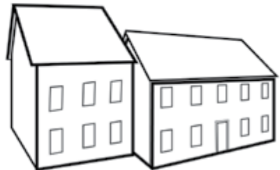
EXISTING SINGLE-FAMILY HOUSE AND ADDITION WITH INCOMPATIBLE MASSING
