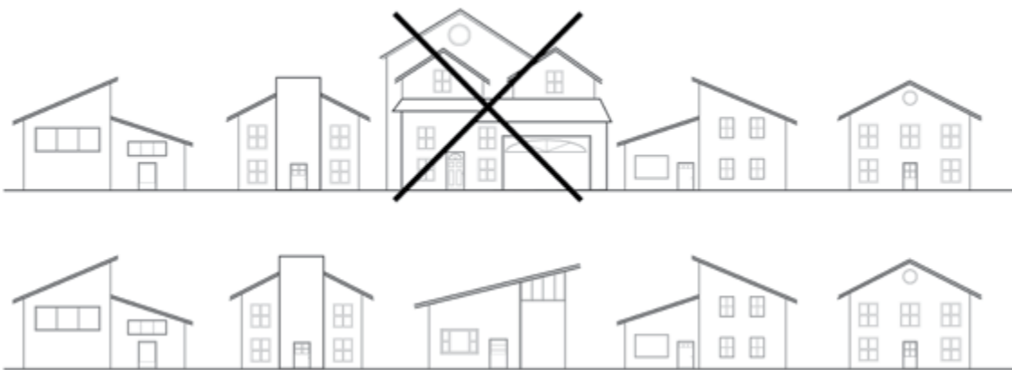
Illustration of a house that is out of scale (top) versus consistent with the predominant scale (bottom) of a streetscape.
